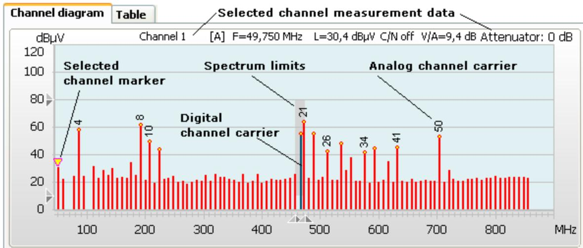
The channel diagram shows a signal level bar display of the selected channel plan or template. The height of the bars corresponds to the signal level (channel power for digital, video carrier for analog channels) and their position corresponds to frequency in MHz. Digital and analog channel bars differentiate by colour.
