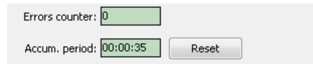
**Reset** button allows to zero the error counter and restart the counting process.
