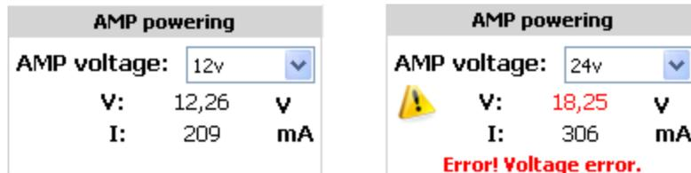
This function is available only for devices supporting the AMP powering function (DAT103). It allows setting the output voltage.
