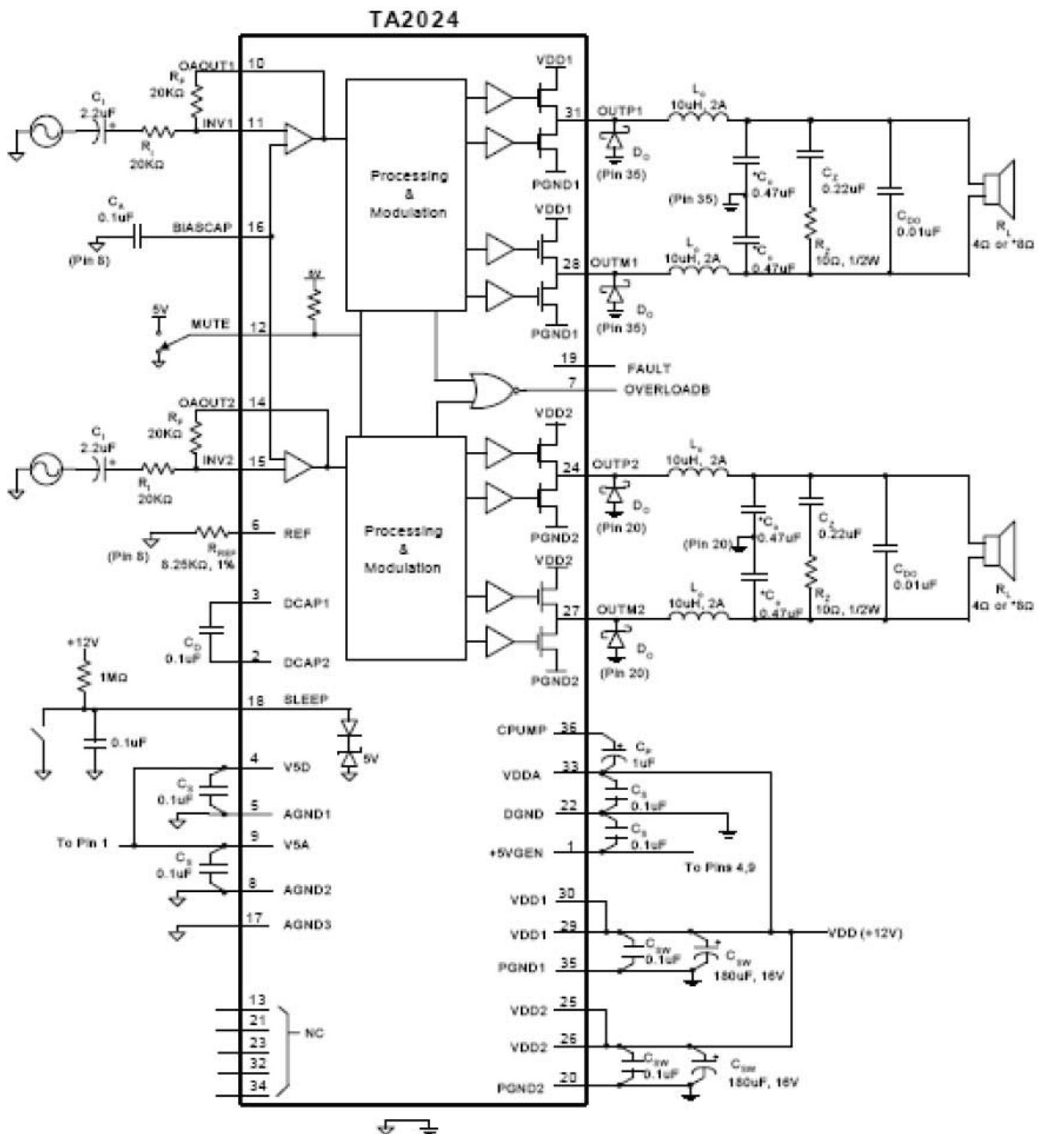
The schematic diagram above is provided for reference. It illustrates the TA-2024 IC and the input and output circuits on the PCB.  $C_{DO}$  are two output capacitors. These capacitors are ideally placed close to the speaker terminals or crossover input terminals as appropriate.
