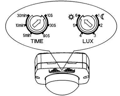
Please note that when testing in daylight, turn the LUX selector to the ☀ (SUN) position, otherwise the sensor will not turn on the load. Also ensure that any lamp connected as a load is pointed away from, and is mounted no closer than 60cm from the sensor.
