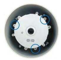
4. Place the camera cover for in-ceiling mount on the camera body and secure the 3 screws with the supplied torx wrench.
