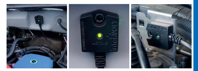
The ISM incorporates a short harness for direct installation to the DCC Pro terminals without need for additional wiring. The device has a single LED indicator which will blink every 8 seconds in standby mode. Once activated by movement the LED will illuminate continuously.
