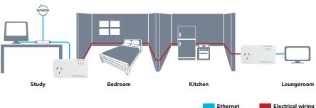
Ethernet Electrical wiring
