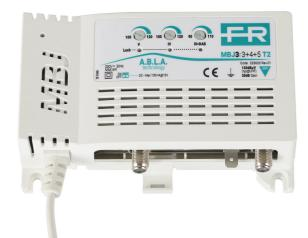
1-input (III+DAB+IV+V) multiband TV indoor amplifier with 35dB gain and up to 120dBµV output level on UHF band, separate bands amplification with independent level adjustment (20dB) for each band and low noise figure. T2 technology with UHF cut band for LTE 4G @790MHz and 5G @694MHz.
