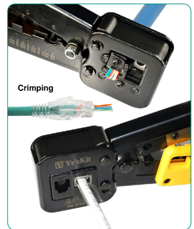
Photo shows boot is crimped with plug and cable, locked as one piece.
