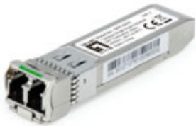
1.25Gbps Single-mode Industrial SFP Transceiver, 80km, 1550nm, -40°C to 85°C SFP-4270
