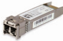
10Gbps Single-mode SFP+ Transceiver, 80km, 1550nm SFP-6181
