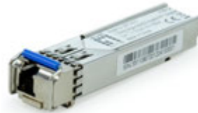
1.25Gbps Single-mode BIDI Industrial SFP Transceiver, 10km SFP-4310
