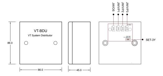
• SET-3Y: Video impedance setting; total 3 settings can be available.75R,150R and HI. 1). connect one BDU. Set to 75R when the distance from door station to BDU is within 50 meters, otherwise set to 150R.(note that set to HI when the video signal is weak) 2).connect multi BDU.Set to 75R when the distance between BDU is within 50 meters, otherwise set to 150R.(note that set to HI when the video signal is weak)
