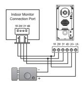
The lock can be directly connected with the door station and the power through monitor. During unlock operation, the monitor will close screen automatically.
