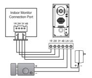
Must install external power supply for lock, and nearly all kinds of electronic lock can be used. Incidentally, in this mode, you can continue talking and monitoring during unlock operation.
