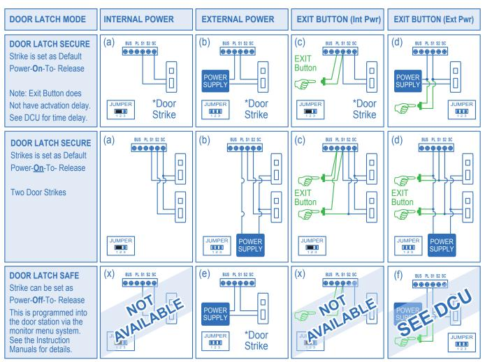
· Fail-Safe / Power-OFF-To-Release type Door Strike Connections
