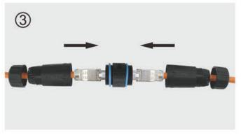
3. Inserting the patch cords into the both ends of the RJ45 coupler.
