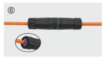
6. Screwing the end cover at both ends onto the long tube. Finally to check whether the waterproof plug is closely matched with the cables.
