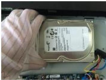
④ Place the HDD in accordance with the four holes on the bottom of the chassis.
