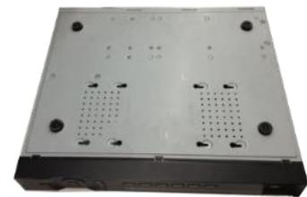
③ Turn the device upside down and then secure the screws firmly. It is to fix the HDD on the chassis.
