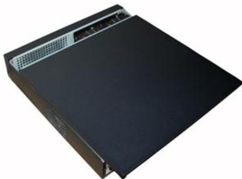
⑨ Secure the HDD bracket and put the top cover back.
