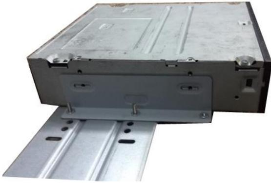
⑤ Install SATA burner. Line up the SATA burner to the hole positions.
