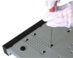
⑤ Turn the device upside down; fix the screws to secure the HDD on the bottom of the chassis.
