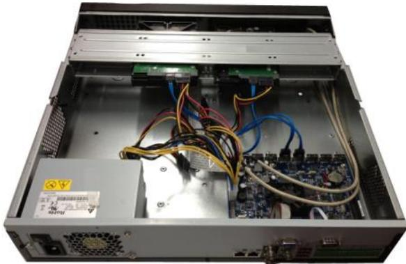
the chassis and then line up the four screws to the four holes in the HDD. Use the screwdriver to fix the screws firmly to secure HDD on the HDD bracket
