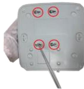
① . Loosen the screws of the bottom of the chassis.
