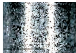
Figure 6 The inner surface of the alloy sleeve before operation and the inner surface of the alloy sleeve after 8,000 hours of operation in 70°C test environment, showing a run-in polishing effect by ceramic shaft
