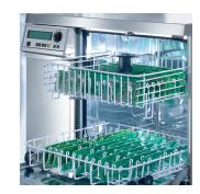
Cleaning processes can be referred to as batch or in-line processes. Batch systems refer to a batch of PCBs taken through the entire process, whether it is ultrasonic or dishwasher application, for example. Cleaning processes can also be set up as in-line systems where PCBs are constantly transferred through each stage and a continuous production line is formed.
