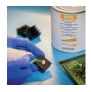
Thermally conductive pastes consist of thermally conductive fillers in a carrier fluid. Thermal pastes do not cure; therefore, they offer the best solution when rework is important and provide versatility by avoiding geometrical restrictions affecting cure.
