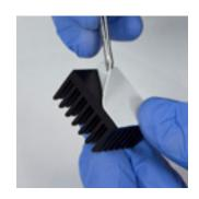
Thermal gap pads are used in place of traditional thermal interface materials (TIMs) such as a thermal paste or RTV. The main benefit of gap pads is that they offer a quick and easy application method, requiring minimal training for the operator and without the mess sometimes associated with a paste, grease or bonding product. In addition, they do not require the use of expensive dispensing machines and can easily be applied via a manual process.
