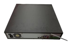
① ①Use the screwdriver to loose the screws
