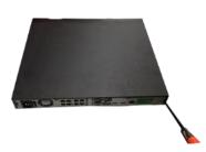
① Loosen the screws of the rear panel and side panel.
