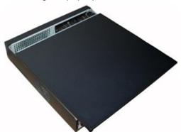
9 Secure the HDD bracket and put the top cover back.
