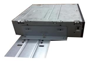
(5) Install SATA burner. Line up the SATA burner to the hole positions.
