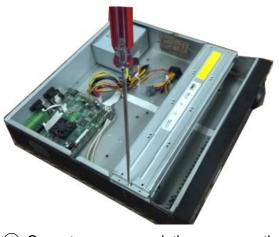
(1) Open top cover and then remove the HDD bracket
