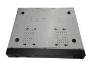
③Turn the device upside down and then secure the screws firmly. It is to fix the HDD on the chassis.
