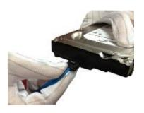
③ Connect the other end of the HDD data cable and the power cable to the HDD.
