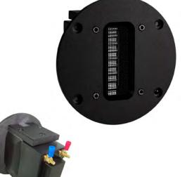
In the correct signal environment, Ribbon tweeters will excel for many years. However, Warning: Ribbon tweeters will destruct with DC and low frequencies. The soft aluminium ribbon will distort itself out of the flux channel and no longer function. Be very cautious. It is recommended to use a high slope crossover filter to protect the tweeter from low frequency and to test your circuit with another tweeter before committing the ribbon to signal. You have been warned.
