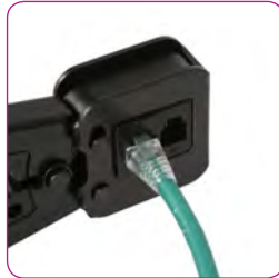
Insert the now assembled plug into the HT346 firmly.
