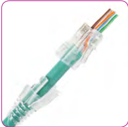
Push the cable through so the wires protrude and the cable jacket is well within the shell for crimping.
