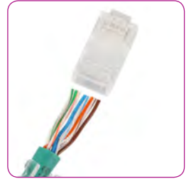
Un-twist and place wires FLAT and in correct order.
