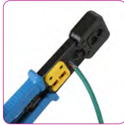
Strip off cable jacket using a wire stripper.
